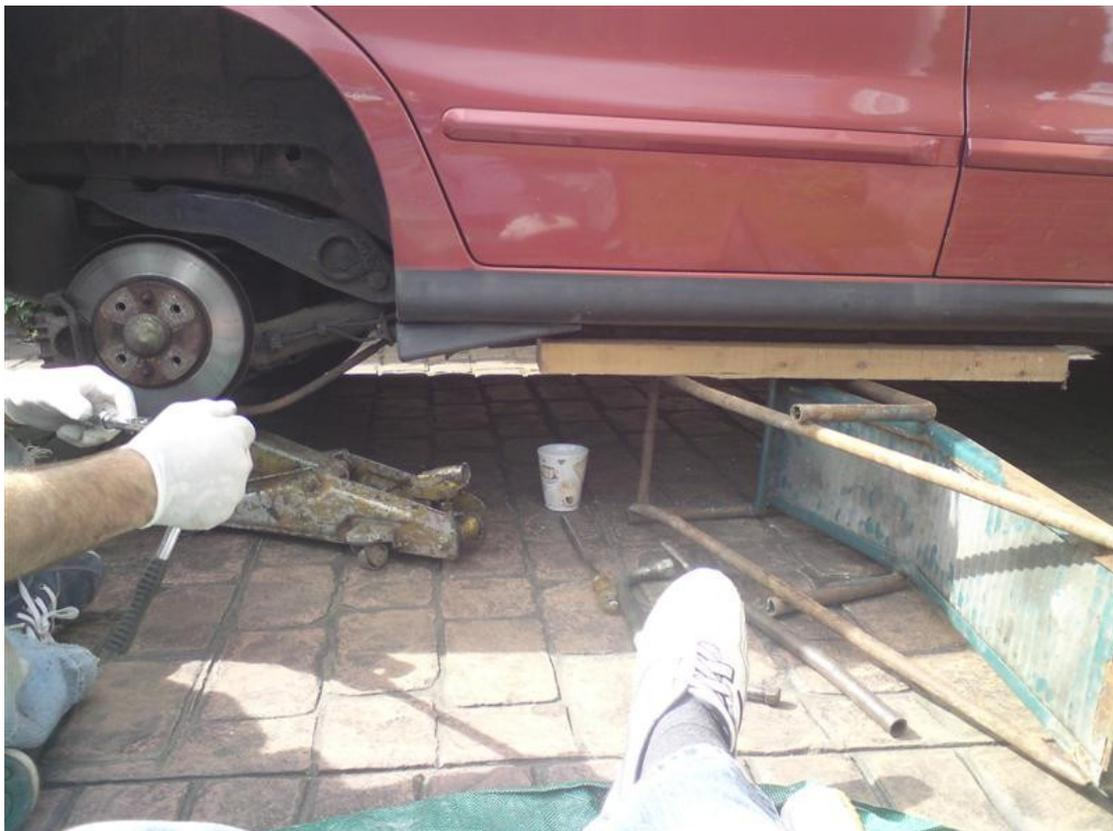
Once in the air use the jack to lift the suspension slightly to make the shock easier to remove.
