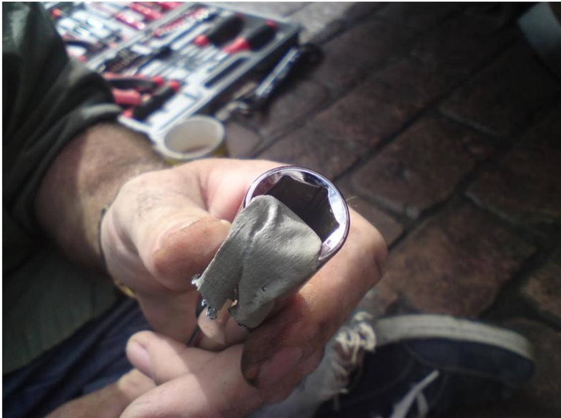
6. Insert the socket and undo the bolt, be careful not to drop it in into the chassis! This is why you need a 'deep' socket...
