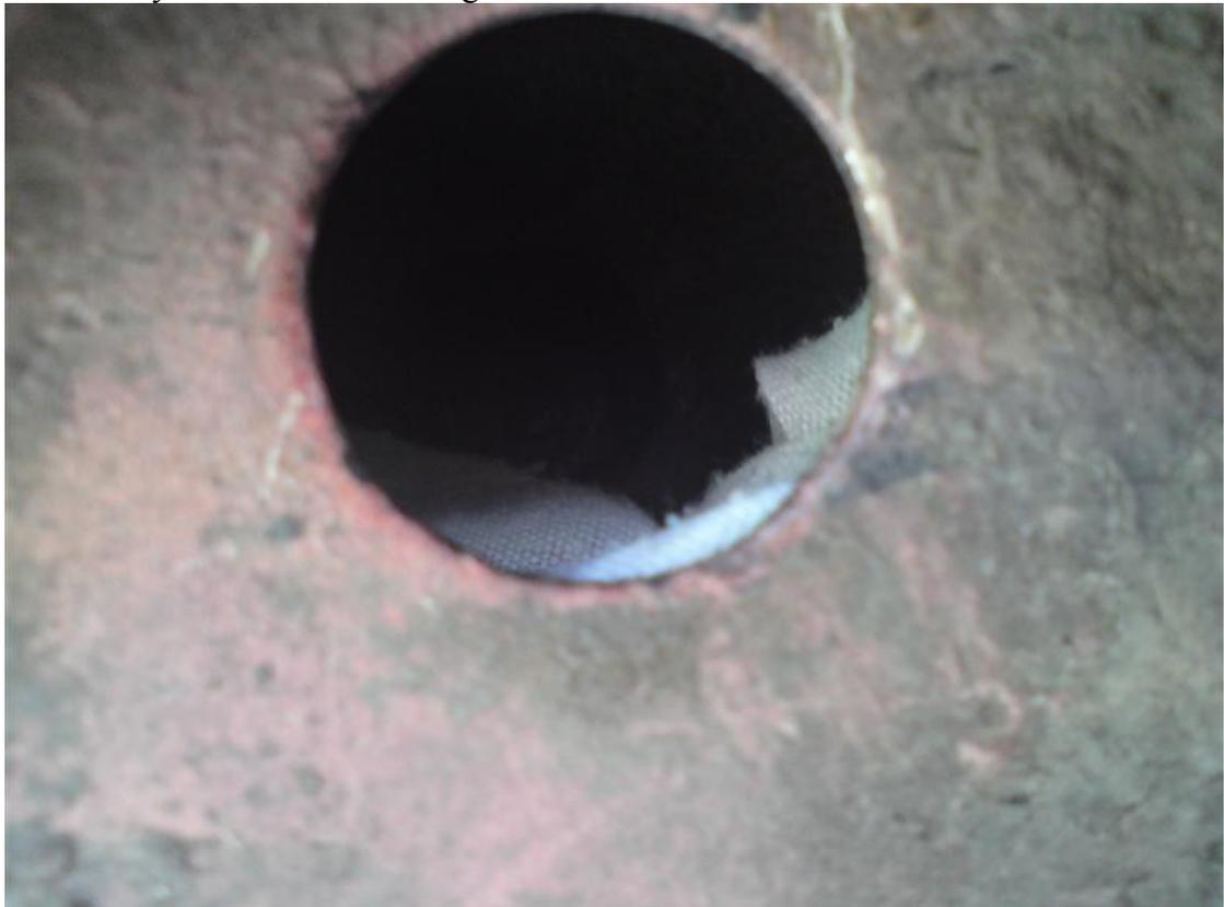
5. Put a bit of folded over Gaffer tape inside the socket to help grip the bolt as it comes out.
