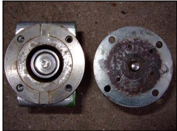
Once you are satisfied the EGR valve is clean and moving freely, put the EGR valve back together, making sure to refit the gasket between the electronic and mechanical parts.
