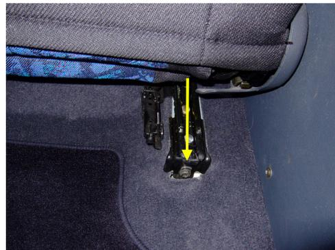
Now put the seat back into its normal position and slide the seat all the way back. Unscrew the two forward mounting bolts as shown. (Alan Key Fitment)
