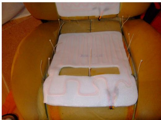
Carefully tilt the seat covering back over the cushion, pay attention to the front of the cushion so that it doesn't rise or move out of place. Make sure there are no folds or bends in the heater elements then start attaching the cable ties to the metal rods in the cover. Working left to right. Make sure the cover is stretched over properly and the strut rod sits in the crevice. Pull the cable ties tight, then cut off any excess, keep working your way back till all seven are done.
