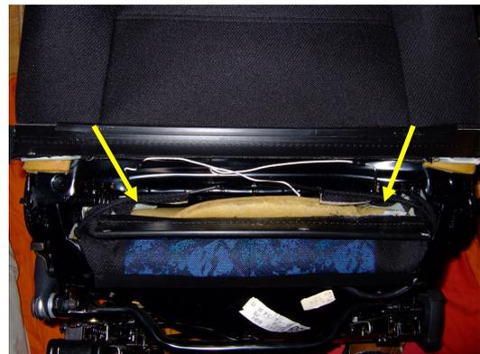
Now clip the two plastic clips from both ends of the cover (front and rear), so that they are perfectly reattached.
