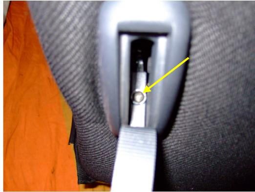
To remove the lever, pull the lever sideways. It will then slide off the metal arm.
