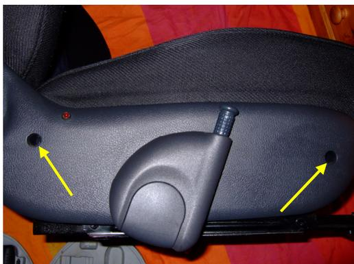
Next unscrew the two remaining self-tapers from the plastic trim. If you have heated seats then disconnect the LED plug under the seat. Now carefully remove the plastic trim. The height adjustment handle does not require removing.
