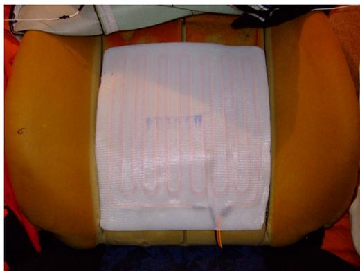
Make sure the upper heating pad has some slack when it is tucked to the right corner, then pull it gently through under the lower foam cushion and connect it to the lower heating element. Feed the power cables through the hole in the seat. Cars fitted with heated seats will have a rubber ring around the hole; if yours does not, then try using some insulation tape to prevent the cable rubbing the sharp edges.
