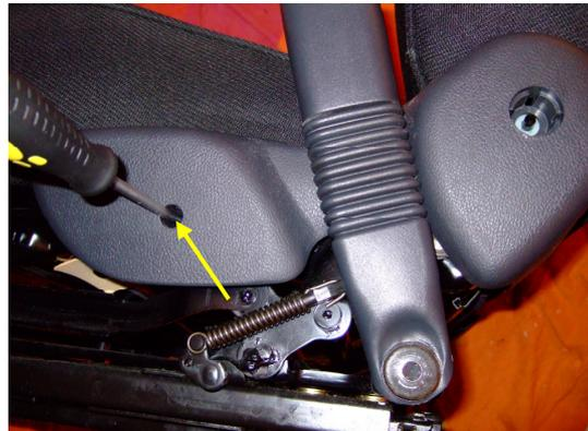
Before the plastic trim can be removed totally you need to carefully place a large flat headed screw driver behind the plastic trim to help push out the metal retaining washer by pushing the trim away from the seat.
