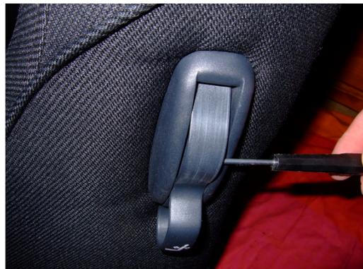
Pull the flap back from the lever to gain access to a hidden screw. Unscrew the screw as shown and withdraw the lever.
