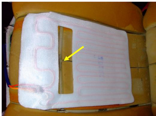
Once you are happy with the way the element is seated, get a screw driver and push a hole through the cushion directly where the wires exit the heating elements at an angle to the thinnest part of the foam cushion. Then use a sharp knife to make a 1.5cm gap then carefully feed the wiring through the hole. As can be seen in the photograph.
