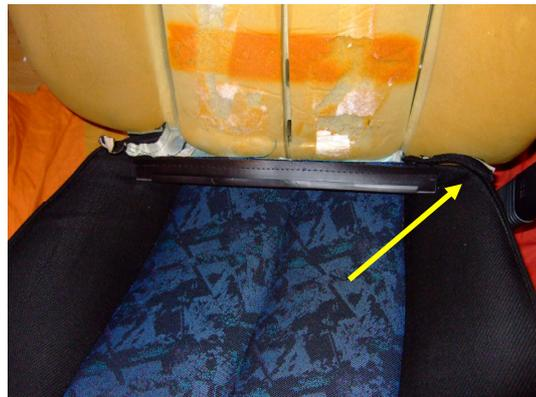
Starting at one corner, as shown by the yellow arrow in the previous photograph; lift this corner up to find a hidden metal ring clip. Be very careful, that you only cut off the metal ring clip and not the metal rod and remove it. Repeat for the other corner.
