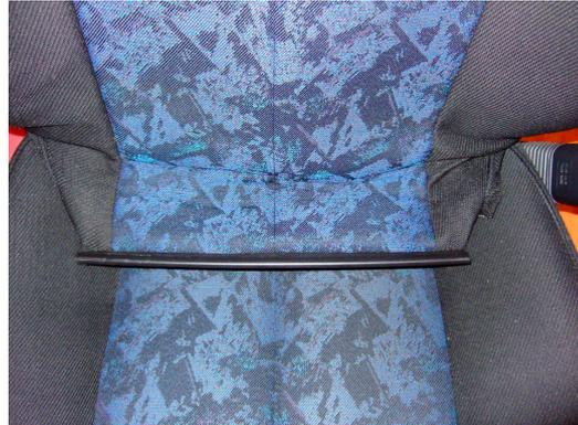
Start by lifting one corner up a little at a time while constantly swapping sides so it evenly starts to rise up the seat. Compress the bolsters to help lift up the cover. The cover will only go approx 2/3 of the way up until the internal seat hooks prevent it from going any further. That is okay, we do not need to go any further.
