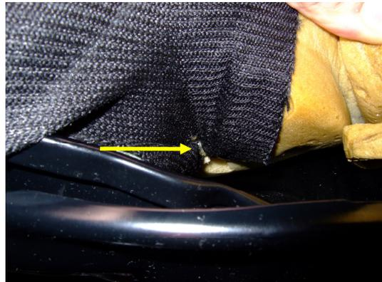
Now the hard part before you can begin to start removing the cushion cover you need to unhook the cover from the sides of the seats. This can be tricky, so again be patient and don't butcher anything. Use a screw driver to unhook the plastic edging on the cover from the frame. Work from the back to the front along the side. Do not carry on unclipping the front, it is not required. Repeat for the other side.
