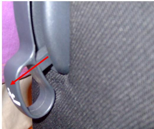
Two further hidden screws will now be revealed, use a screw driver to remove them and then carefully remove the handle surround away from the seat.
