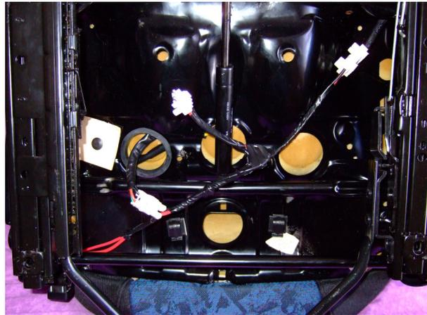
This is how I have currently set up my seats; if you prefer to use the wiring loom that came with the heating elements, just connect the orange and red wire to either of the red/green wires from the vehicles own wiring under the seat and the negative wire to either black wire under the seat.
