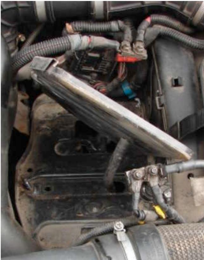
You are now left with the battery tray and its plastic tray on it. So you have to remove the plastic tray, to do so, just lift it up like on the picture left.
