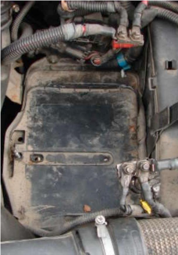
Now remove the tin holder that the nut tightened and also remove the strap that goes over the battery. After that done, take out the battery.
