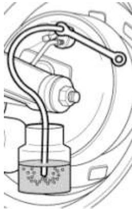
Now you are left only with the tin battery tray. Looking on it, you will see it has 2 cut out holes; the upper one is access for bleeding the slave cylinder.
