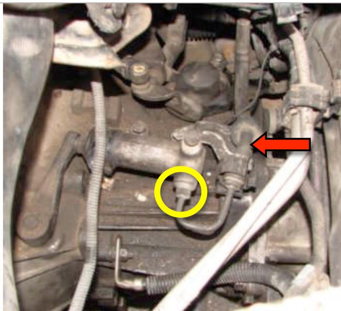
To remove the old cylinder and put on a new one, you have to clamp the incoming rubber hose (red arrow) using a clamp or pliers like on the picture left.
